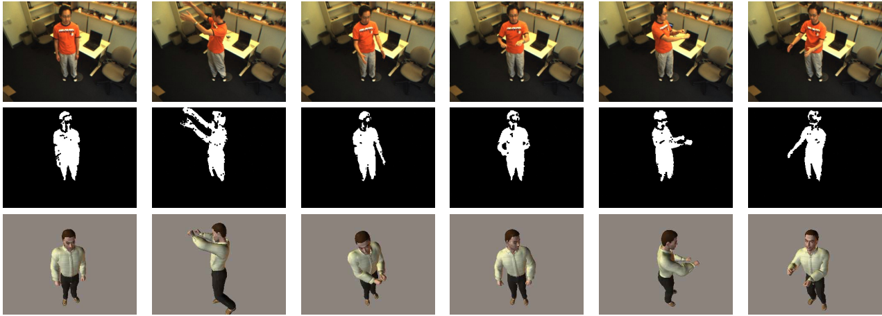
Figure 4: Sample frames from a gesture sequence (first row), segmentation masks (second row) and the corresponding frames from a most likely sequence computed by CRPV algorithm (third row).
