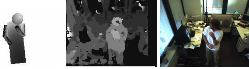
Fig. 2. Our geometric-based tracking algorithm minimizes the Euclidean distance between an articulated model (left image) and the 3D reconstruction of disparity image (middle image) corresponding to the scene (right image).
