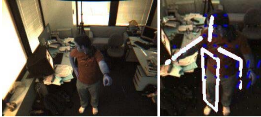
Fig. 1. The left image shows the current image. The right image shows the detected key frame of the view-based model, optical flow of the support points (in blue) and the prediction of the articulated body pose from the linear model (in white).
