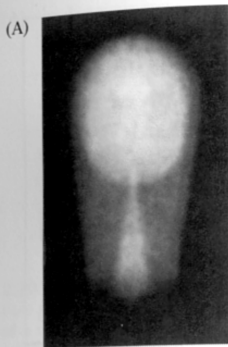
2.18 DIFFRACTION LIMITS THE QUALITY OF PINHOLE OPTICS. These three images of a bulb filament were made using pinholes with decreasing size. (A) When the pinhole is relatively large, the image rays are not properly converged, and the image is blurred. (B) Reducing the size of the pinhole improves the focus. (C) Reducing the size of the pinhole further worsens the focus, due to diffraction. From Ruechardt, 1958.
