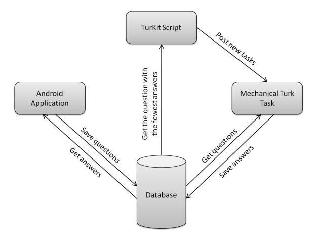
Figure 4-1: The four major components of the Sinch system architecture.
