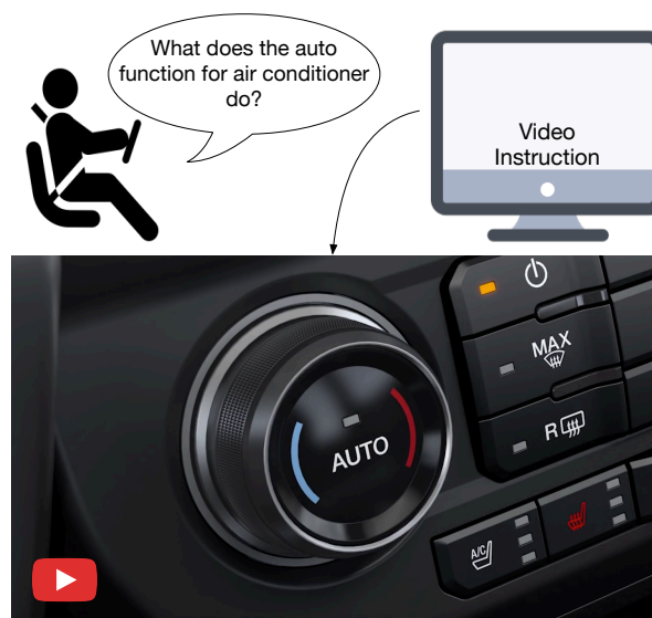
“the system also comes with an auto function it automatically controls the temperature air distribution and air flow to reach and maintain a comfort level based on the temperature you selected”
