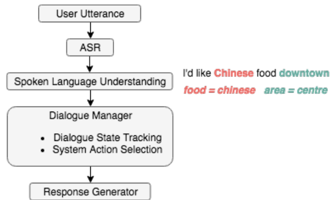
Fig. 1. The typical flow of a dialogue system, with spoken language understanding followed by dialogue state tracking.
