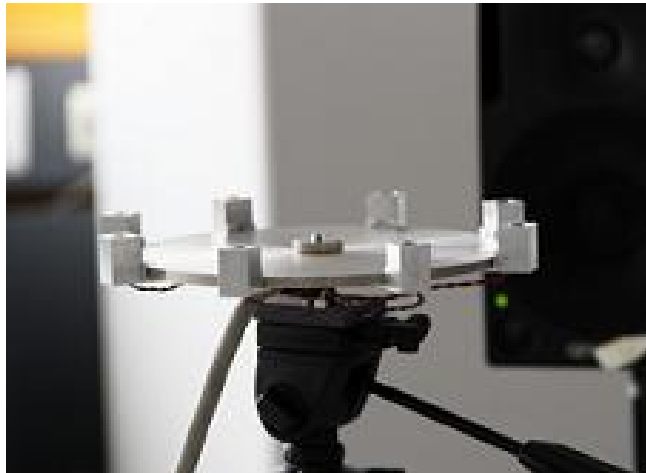
Figure 3-5: 8-channel microphone array used in the reverb challenge dataset
