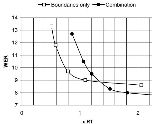
**Figure 2.** Word error rate versus computation for the boundary/segment model combination (with 10 mixtures per segment model) compared to the boundary models only system. Timing performed on a 500MHz Pentium III.
