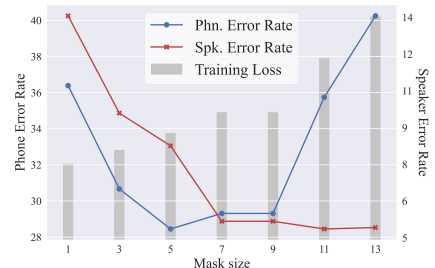
Figure 2: Phone/speaker error rate and training loss with respect to different mask size on 2-layer NPC with R = 23 .
