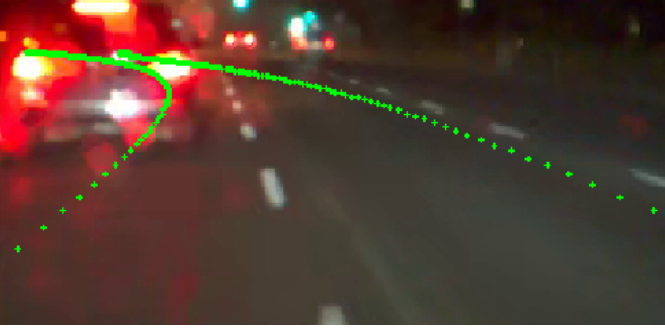
Fig. 5: An example of a lane-detection failure detected by the monitor. The green lines represent the proposed lane lines.
