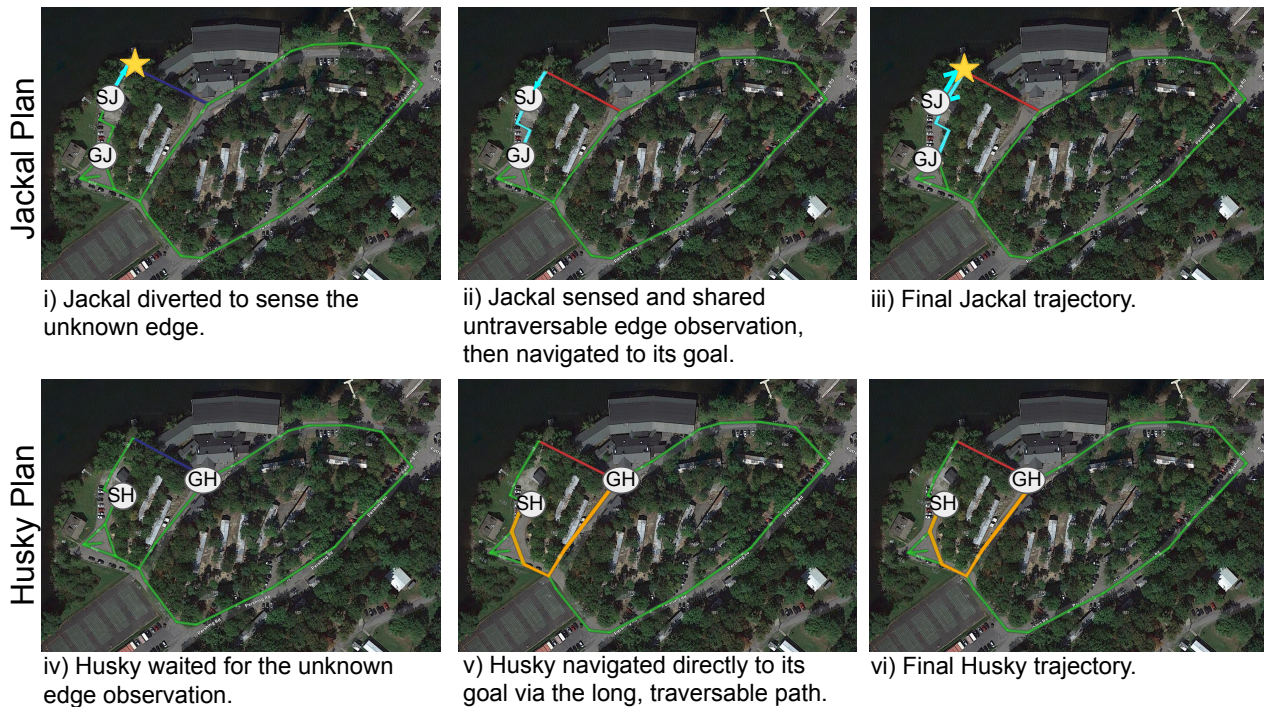
Fig. 6. a) Graph-based plans selected by the non-collaborative baseline planner, visualized over the abstract navigation graph. The Jackal (blue) with start SJ and goal GJ navigated directly to its goal, while the Husky (orange) with start SH and goal GH navigated to the unknown edge, sensed that it was untraversable, and then backtracked to the goal via the long, traversable path. b) Graph-based plans selected by the collaborative planner, visualized over the abstract navigation graph. The Jackal (blue) with start SJ and goal GJ diverted to the gold star to sense the unknown edge, and shared the untraversable edge observation with the Husky. Then, the Jackal navigated to its goal. The Husky (orange) with start SH and goal GH waited to receive the edge observation from the Jackal, then navigated directly to its goal via the long, traversable path. Note that some trajectories were hand-annotated from raw agent outputs for clarity and due to agent/ground station communication drops.
