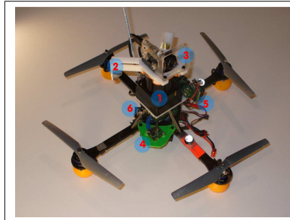
Figure 1: Our quadrotor helicopter. Sensing and computation components include a Hokuyo Laser Rangefinder (1), laser-deflecting mirrors for altitude (2), a monocular camera (3), an IMU (4), a Gumstix processor (5), and the helicopter’s internal processor (6)
