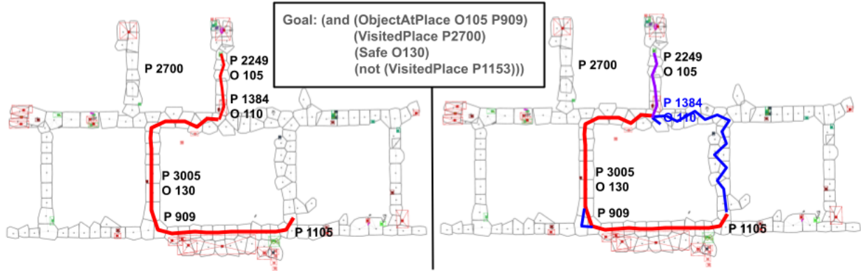
Figure 5.3: A visualization of a high-level plan derived from our Direct encoding, attempting to solve a subset of a task specification in the MIT building 45 environment. On the left we see the first plan proposed by the high-level PDDL planner. However, this plan is obstructed by O110 , and so we must consider different plan skeletons. Because the task planner cannot be certain if a different sequence of Move actions might lead to success, we may have to consider many different abstract plans before attempting one which moves the obstruction out of the way. On the right, we highlight a few such superficially different plans.
