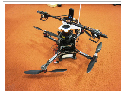
Figure 2. (a): CAD drawing of the quadrotor design with simulated fields of view. (b): final assembled quadrotor with stereo camera system, laser range-finder, WiFi dongle and on-board computer
