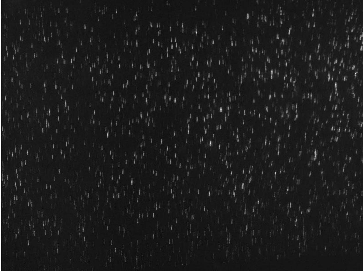
Figure 5-1: A sample frame from Experiment 1's straight and laminar flow.
