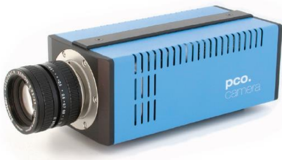
Figure 3-2: Left: The high-QE PCO.1600 camera used for imaging. Right: The LaVision 2 Watt Continuous Wave 532nm laser.
