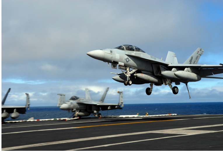
Figure 1-2: An F-18 lands on an aircraft carrier (U.S. Navy, 2008). Notice that the fighter jet lands at a relatively low angle of attack (about 8.1 degrees) in order to avoid stall. The aircraft must be slowed down by a hook and tow cable as it lands.
