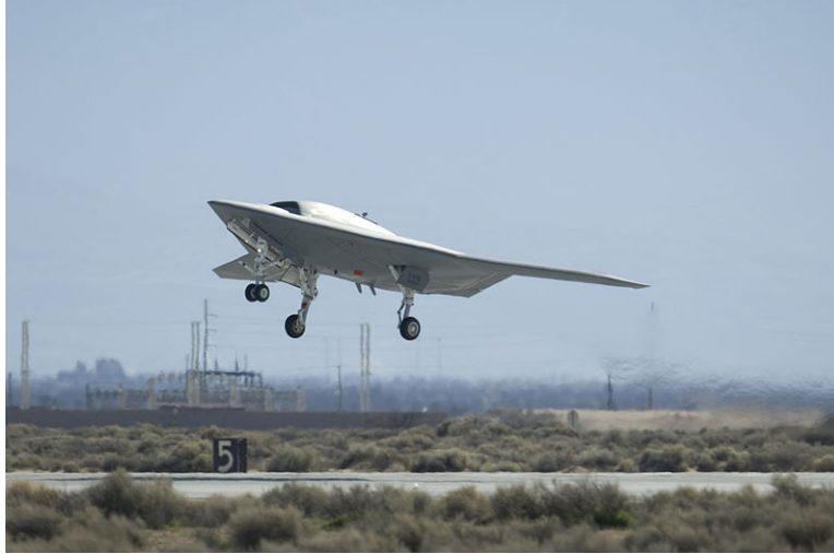
Figure 1-4: A Navy X-47B Unmanned Combat Air System (U.S. Air Force, 2011). Currently, UAVs also must land at low angles of attack to avoid stall. Such unmanned systems could benefit greatly from the development of robust fixed-wing perching maneuvers.
