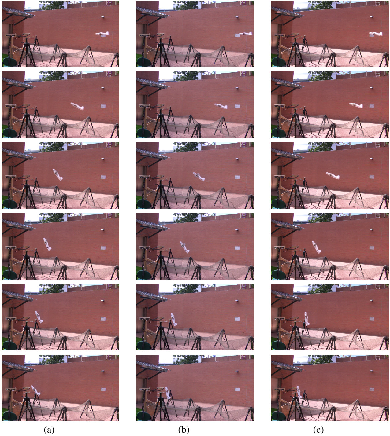
Figure 8-13: These movie stills demonstrate three sequential outdoor perching maneuvers, using only onboard electronics. When there are not any significant winds, perching is successful.
