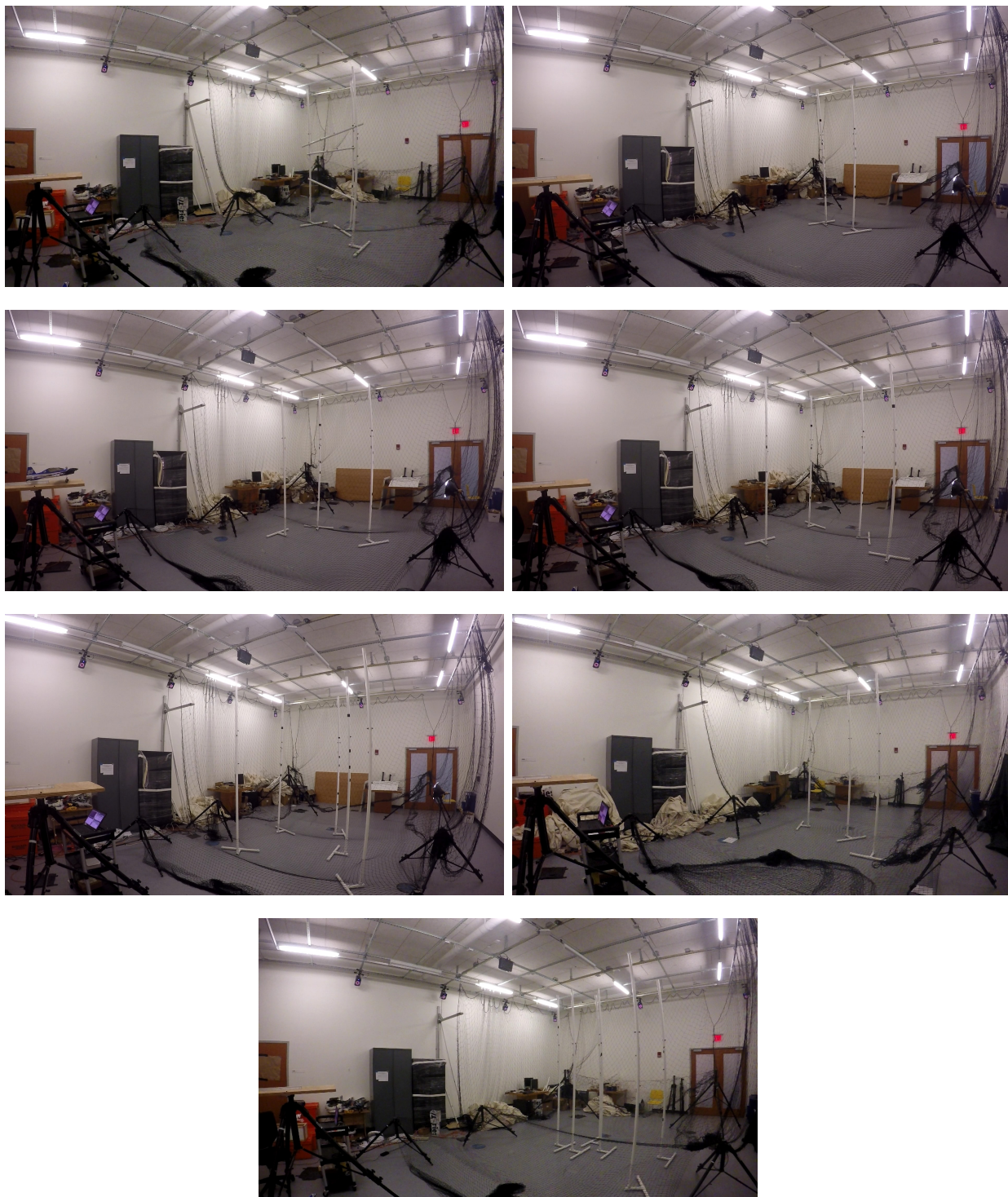
Figure 8-6: Environments 9-15 on which we tested our planning algorithm. The bottom most image shows the only failure case. Here the airplane brushed one of the obstacles on its way across the room.
