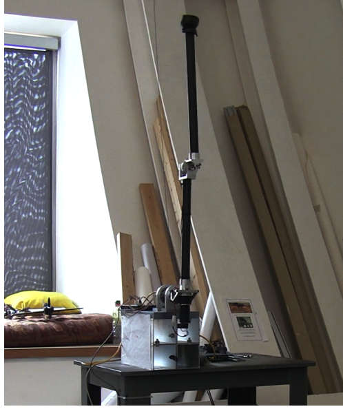
Figure 9-4: Picture of the Acrobot balancing in the upright configuration using the controller designed with SDSOS programming. A video of the controller in action is available online at https://www.youtube.com/watch?v=FeCwtvrD76L .
