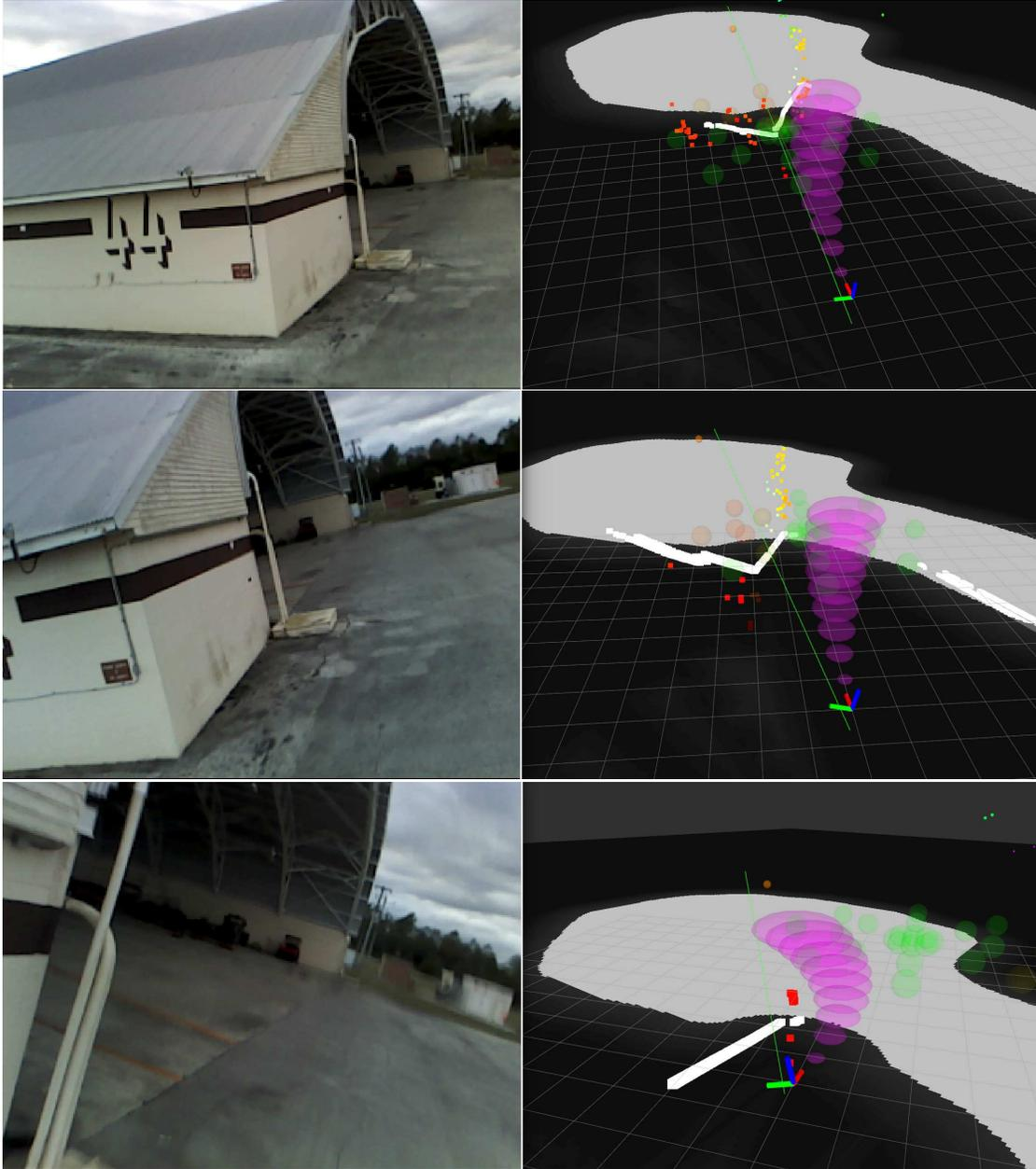
Figure 3-17: Flight at  $7\text{ m/s}$  around the edge of a hangar. With mostly laser returns and only sparse RealSense returns, the vehicle rolls right to avoid the wall (top). Despite a bug in the global planner that caused it to propose bad plans when in false-positive occupied space (middle), the local planner is responsible for navigating the vehicle to safety. As soon as the vehicle has dynamically cleared the wall (bottom), it snaps around it with a left roll.
