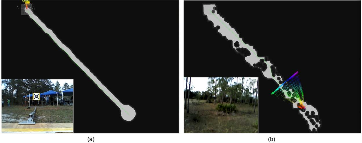
Figure 3-7: Prior map (a) and map on return flight (b). The inset shows an onboard image at the start location pointing north (a), and on the return flight in the forest (b). The 2D A\* global plan is shown in light green. The colored view cone is the FOV of the RealSense sensor, which will give returns out to 60  $m$ , even though only the first  $\sim 10\text{-}20$   $m$  are typically useful.
