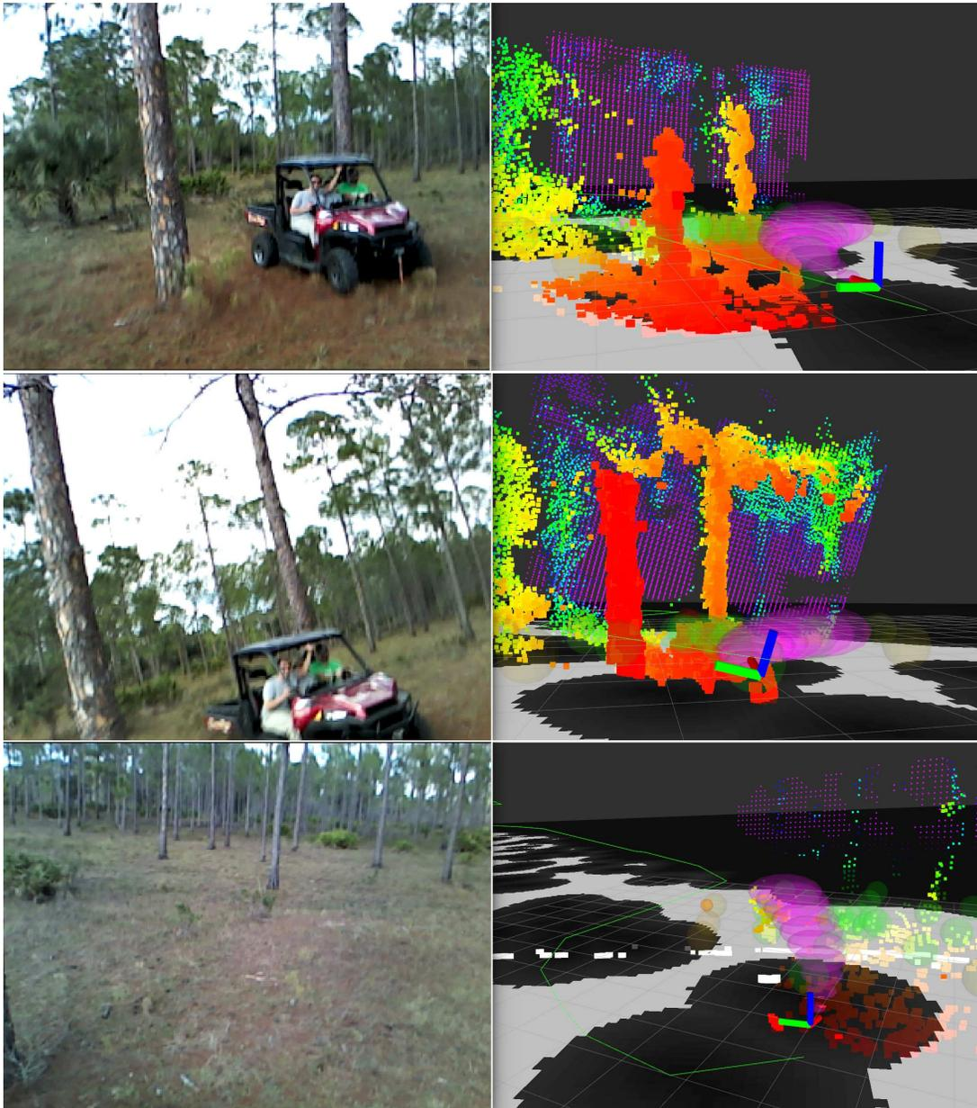
Figure 3-13: Return,  $5\text{ m/s}$  from Flight i. Quadrotor approaches a pair of obstacles (top), not that although the initial velocity is to the right, the A\* planner does not encode dynamic constraints and plans a path to the left. The quadrotor instead dynamically avoids the car to the right, passing the car (bottom) and returning to level flight (bottom).
