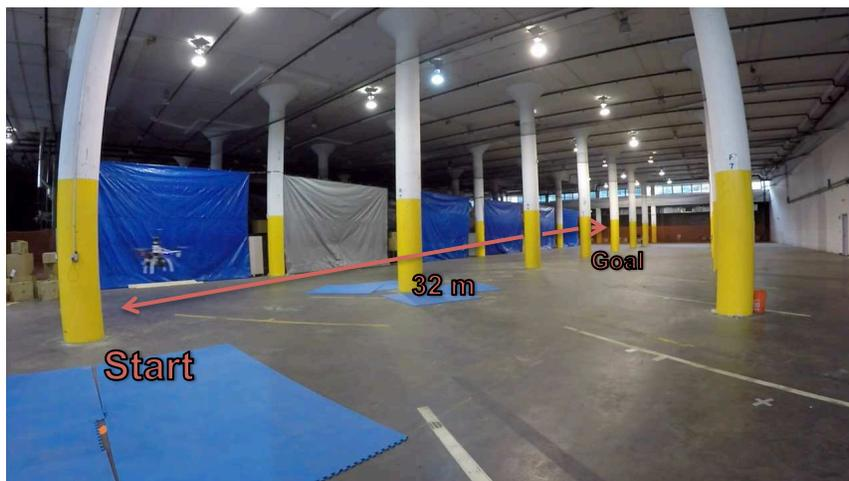
Figure 3-2: Setup of warehouse environment, and locations of start and goal (32 m away, behind the row of pillars).
