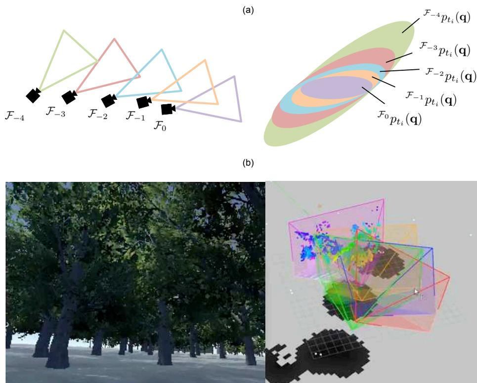
Figure 4-1: (a) Depiction of frame-specific configuration uncertainty  $\mathcal{F}^{-j}p_{t_i}(\mathbf{q})$  for a series of depth image field of views (FOVs). (b) Visualization of using Depth-Pose-Graph Planning to navigate a simulated forest (simulated image on left, visualization of subset of recent FOVs on right).
