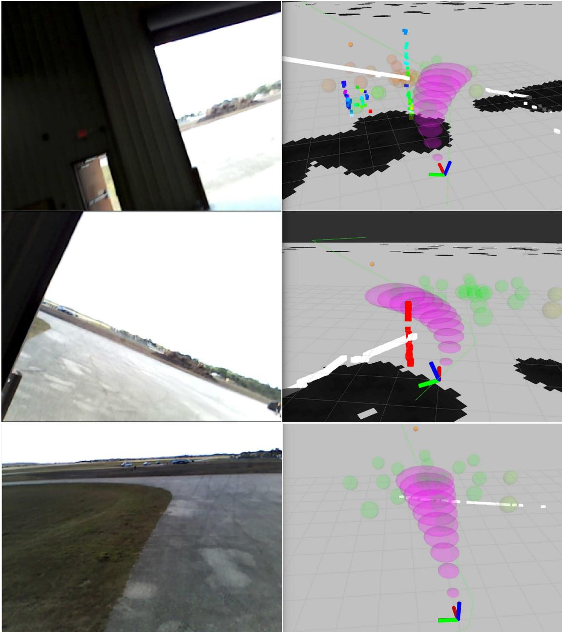
Figure 3-18: Flight at 6  $m/s$  exiting a warehouse to outdoors. The vehicle relies on mostly laser perception (top) to see the opening, then snaps around it (middle), and comes to level flight after clearing the exit (bottom).
