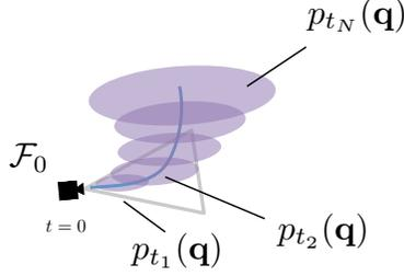
Figure 4-5: In current frame  $\mathcal{F}_0$ , sampling time-varying distribution of configuration at times  $t_1, t_2, \dots, t_N$ . The FOV of the depth sensor is shown with the gray triangle.
