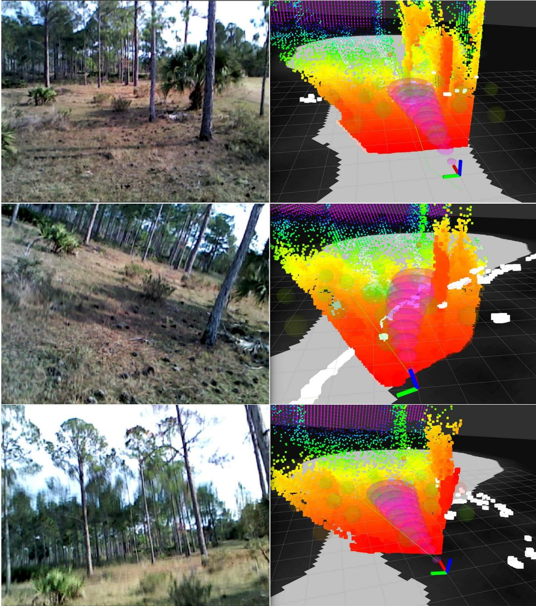
Figure 3-12: Outbound, 5  $m/s$  from Flight i. Vehicle approaches a pair of trees (top), rolls left 21.2  $deg$  and then rolls right out of the dodge (middle), and returns to forward flight (bottom). Note that although the global plan veers off to the left due to mapping errors, the local planner chooses to fly through the open.
