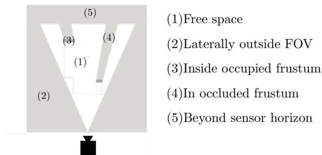
Figure 4-3: The five subsets of space partitioned by one depth image.
