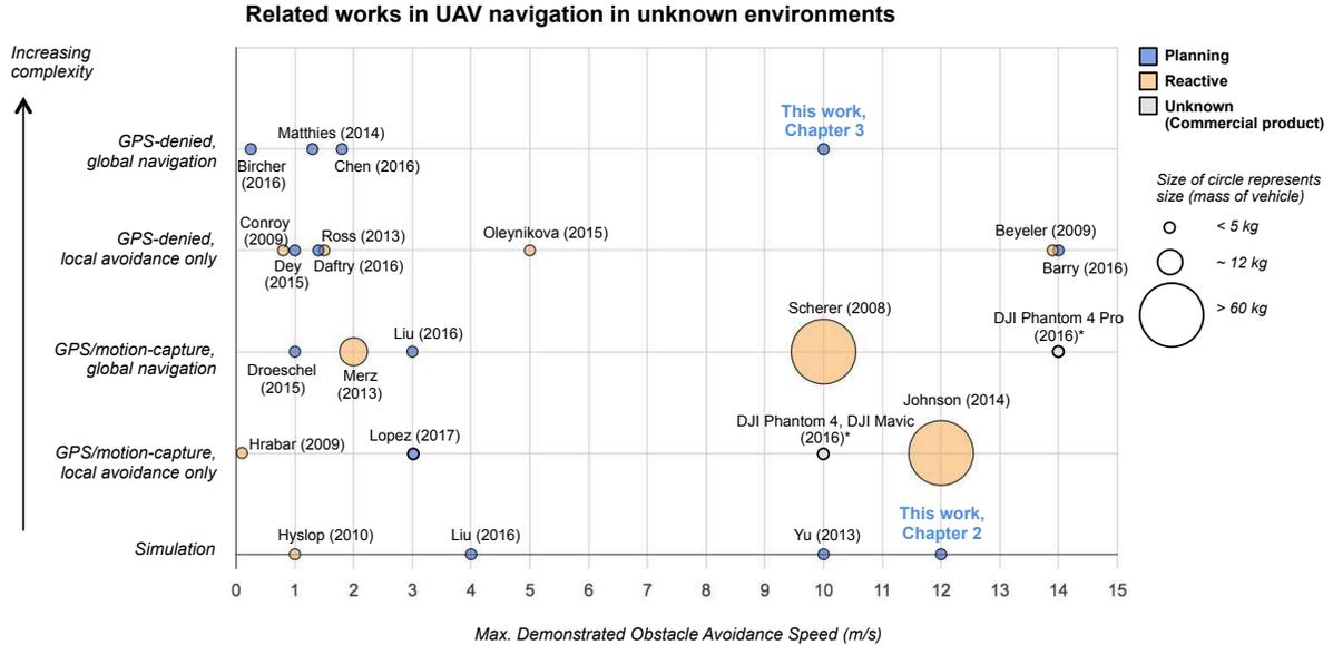
Figure 1-7: Comprehensive comparison of works in UAVs navigating unknown environments that meet the requirements stated below. Asterisk \* denotes that the numbers are reported for manual-pilot obstacle assistance, and may be different for fully autonomous navigation.
