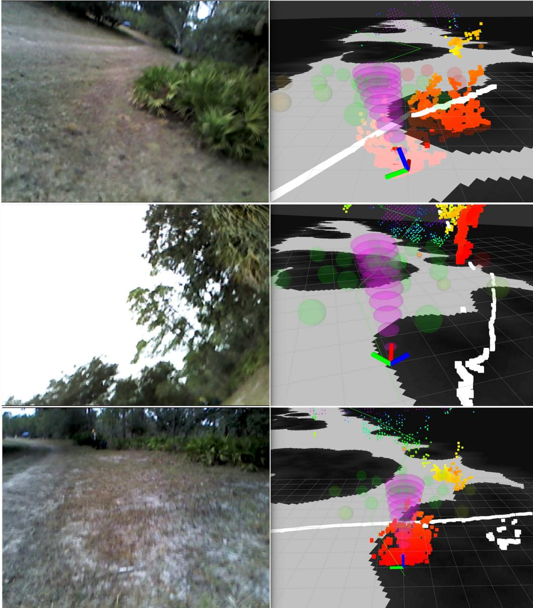
Figure 3-16: Outbound, 6  $m/s$  from Flight iii. Vehicle approaches shrubs and rolls left around them (top), snaps around the corner with a 44.2  $deg$  roll (middle), then returns to level flight (bottom).
