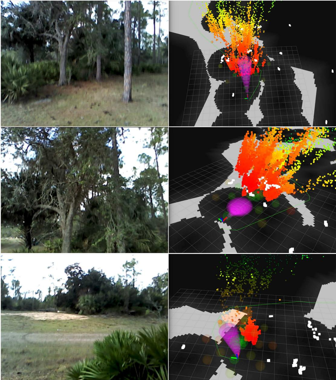
Figure 3-14: Demonstration of the global planner helping the vehicle get out of a dead end. The vehicle approaches a dead end (top) at 5  $m/s$  (Flight i), chooses to stop to avoid collision (middle), and the global planner then guides the vehicle around to the left, out of the dead end (bottom).
