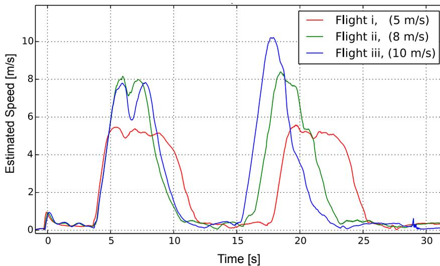
Figure 3-3: Speed over time for the three warehouse flights. When the vehicle speed is near 0, it is turning around at the goal.
