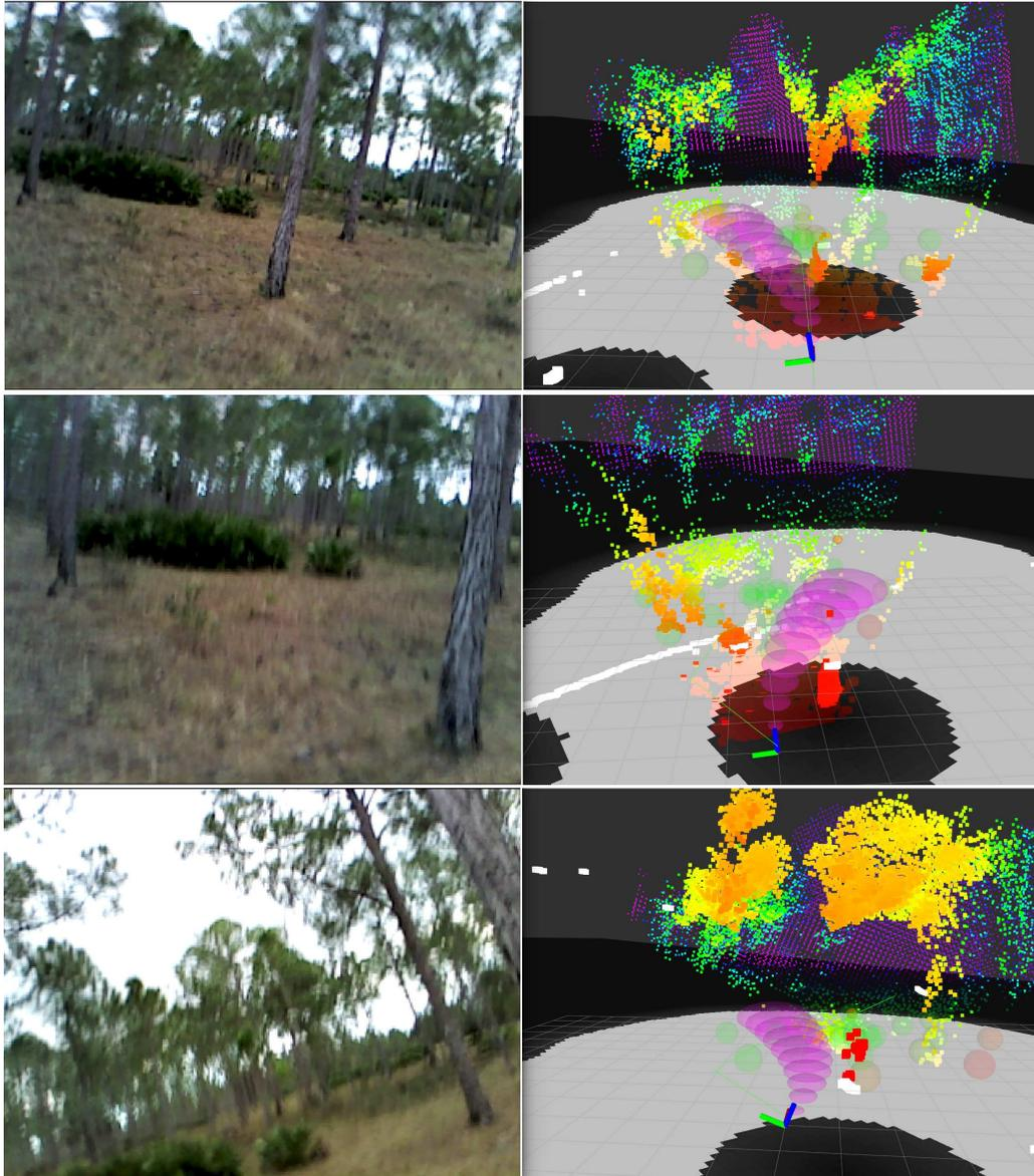
Figure 3-15: Outbound, 6  $m/s$  from Flight ii. Vehicle approaches tree (top) and rolls to left, then chooses to snap around tree as soon as it is safely past (middle), rolling 28.9  $deg$  as it comes around (bottom).
