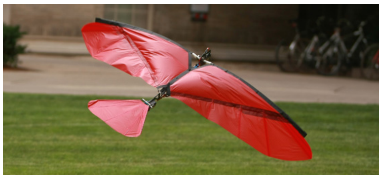
Figure 7-5: Our Phoenix ornithopter. This robotic bird carries an embedded computer running linux in its belly, with gyros, accelerometers, magnetometers, and sonar sensors all on board. Communication is done through an on-board wi-fi access point. Design by Zack Jackowski.
