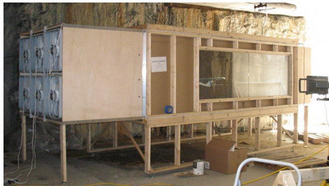
Figure 7-2: Actual pictures of our free flight wind-tunnel.
