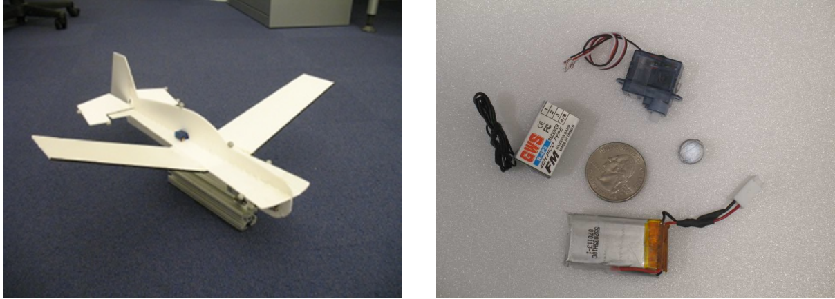
Figure 3-1: (left) Our experimental glider with a 20^\circ dihedral on the wings for passive lateral stability. Reflective markers are placed along the body and the elevator in order to reconstruct absolute position and orientation using the Vicon motion capture system. (right) Electronics and components: (clockwise from top) hobby servo, motion capture marker, battery, micro receiver. (Quarter shown for scale).
