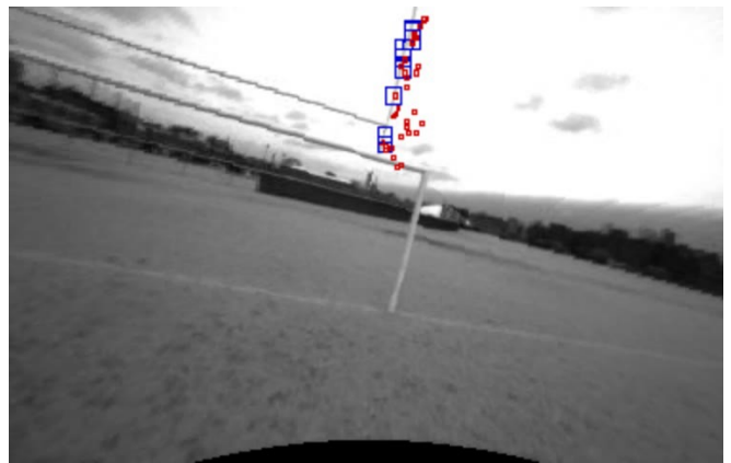
(b) Obstacle detections with the pushbroom stereo system. Detections generated by this frame are in blue and past detections reprojected onto the frame via the state estimate are in red.
