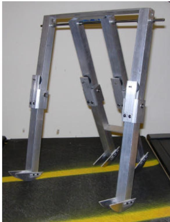
*Figure 4-1: Picture of walker based on McGeer's design*
