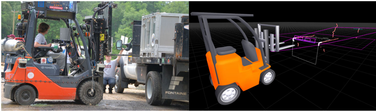
Figure 7. The robot detects the presence of the truck bed and pallet and maintains estimates of their geometry throughout engagement using LIDARs mounted to the tines and carriage.
