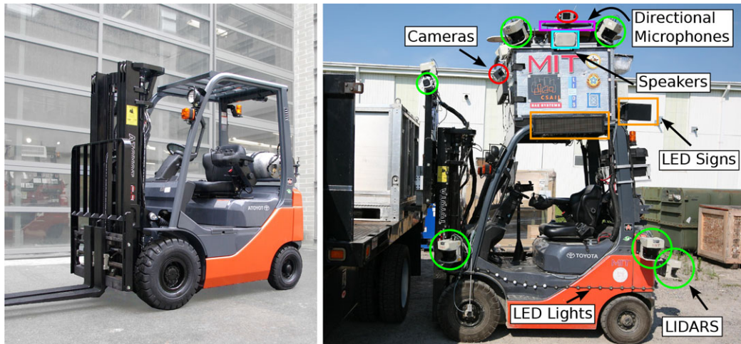
Figure 2. The platform is based upon (left) a stock 2,700 kg Toyota lift truck. We modified the vehicle to be drive-by-wire and equipped it with LIDARs, cameras, encoders, an IMU, and directional microphones for perception; and LED signage, lights, and speakers for annunciation. The compartment on the roof houses three laptop computers, a network switch, and power distribution hardware.
