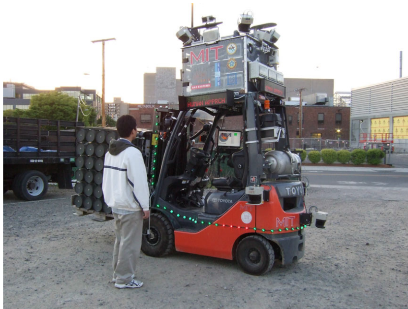
Figure 16. The robot utilizes a combination of LED signs and LED lights to indicate that it is aware of people in its vicinity. The lights mimic the robot's gaze toward approaching pedestrians.
