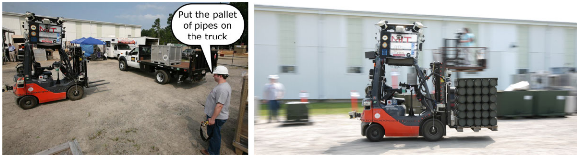
Figure 1. The mobile manipulation platform is designed to safely coexist with people within unstructured environments while performing material handling under the direction of humans.
