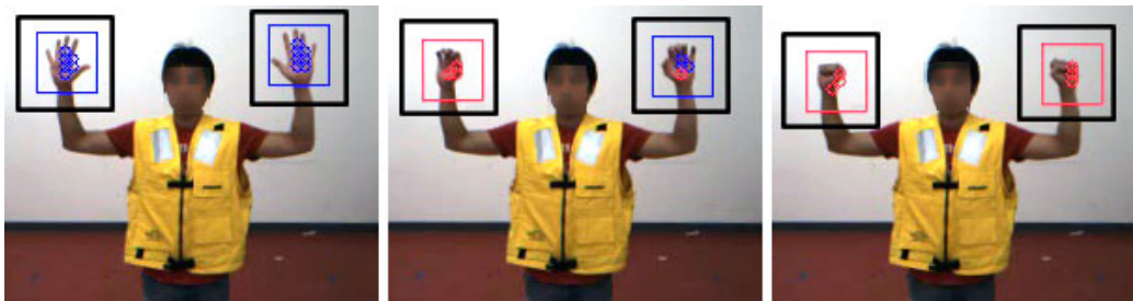
Figure 2-7: Search regions around estimated wrist positions (black rectangles) and clustering of multiple classification results. Our search region was 56 x 56 pixels (outer rectangles); the sliding window was 32 x 32 pixels (inner rectangles). Inner rectangles indicate clustered results (blue/red: palm open/close), and small circles are individual classification results (best viewed in color).
