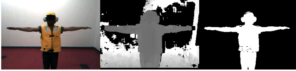
Figure 2-3: Input image (left), depth map (middle), and mask image (right). The “T-pose” shown in the figures is used for body tracking initialization.
