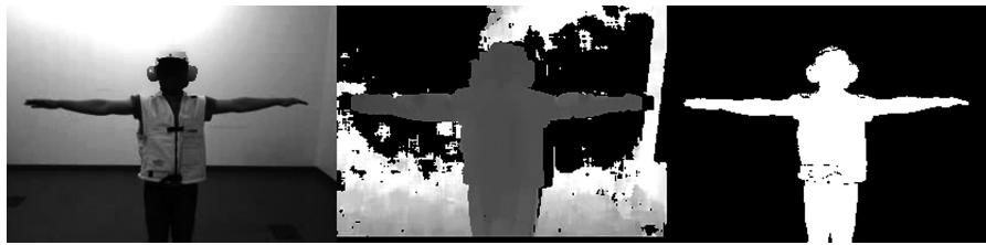
Fig. 2. Input image (left), depth map (middle), and mask image (right). The “T-pose” shown in the figures is used for body tracking initialization.
