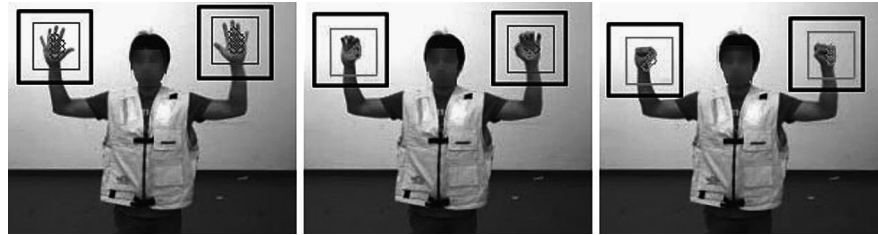
Fig. 6. Search regions around estimated wrist positions (outer rectangles) and clustering of multiple classification results. Our search region was 56 \times 56 pixels (outer rectangles); the sliding window was 32 \times 32 pixels (inner rectangles). Inner rectangles indicate clustered results (blue/red: palm open/closed), and small circles are individual classification results (best viewed in color).
