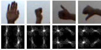
Fig. 4. Four hand poses and a visualization of their HOG features. Bright spots in the visualization indicate places in the image that have sharp gradients at a particular orientation, e.g., the four vertical orientation in the first visualization.
