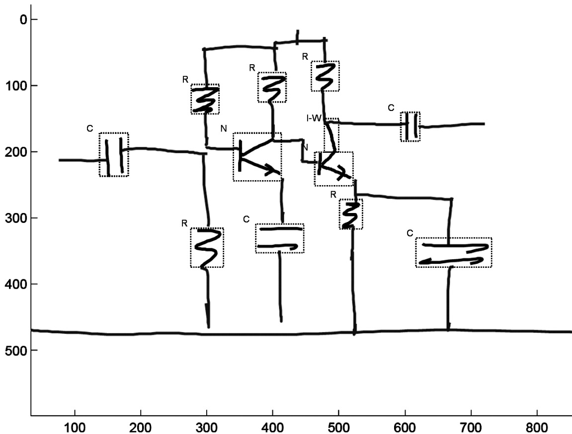
Figure A-1: In this example, the user interspersed a wire connected to the collector of the transistor Q2 . We present a model that can recognize objects correctly even in the presence of such interspersings and identify interspersed objects (indicated by I-W).
