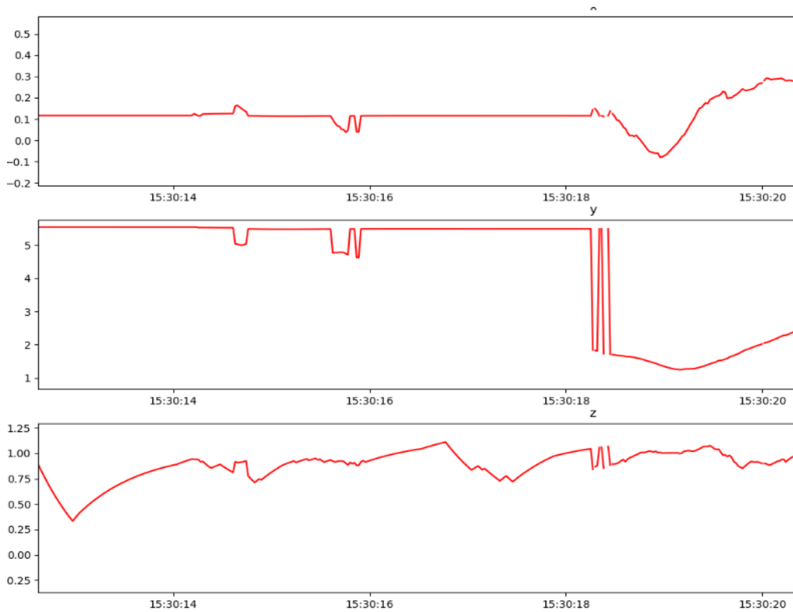
The middle graph shows an example of extreme oscillation between 15:30:18 and 15:30:20.
