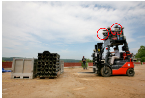
(b) The positions of the front and left cameras are marked in red.
