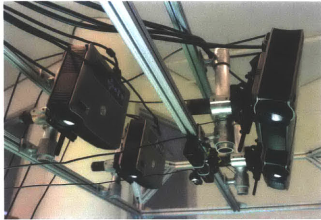
Figure 3-1: An overview of our seamless display hardware. Mounted above the table are 4 projectors, a Kinect sensor, and a webcam. A Windows 7 desktop sits under the table.
