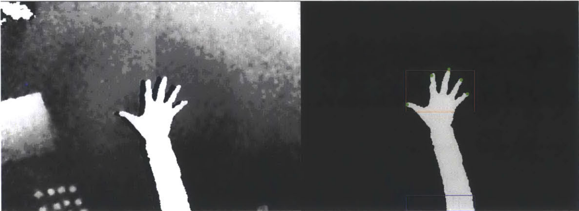
Figure 5-3: Raw depth image shown on left (lighter pixels are closer to camera), final result after background subtraction and finger identification shown on right. The red box shows the hand regions, the blue box shows the forearm region that enters the frame. Green dots are calculated fingertips.
