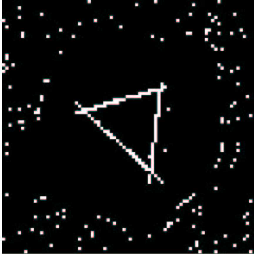
Figure 1: The result of programming the beacon with the design for a structure of three corners, each at equal radius, with 120 degrees between successive corners and straight walls between them. Only bricks and agents embodying corners are shown.
