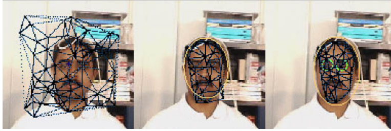
Figure 9: Mesh initialization. The mesh is initially distributed arbitrarily. It is pruned by the head outline when it is detected, and by heuristics based on the relative motion of different parts of the mesh. When frontal pose is detected, surface coordinates of the mesh can be initialized within the parallel region (that part of the face that is parallel to the image plane).
