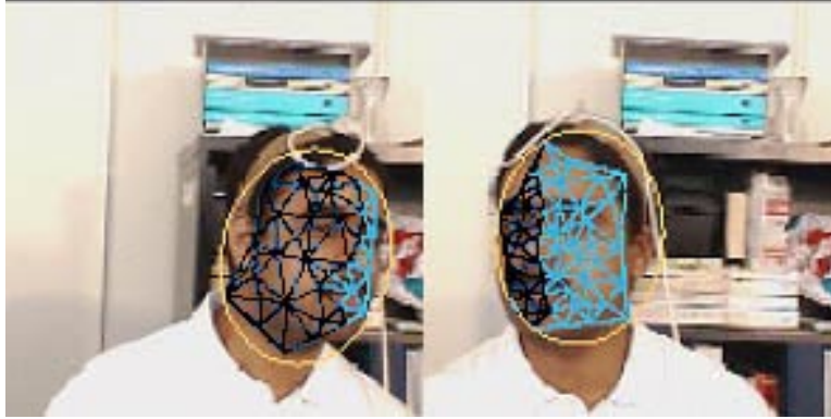
Figure 10: A visualization of surface coordinates on the mesh. The mesh has been colored here based on the sign of a surface coordinate, so that it appears as two halves locked onto either side of the face.
