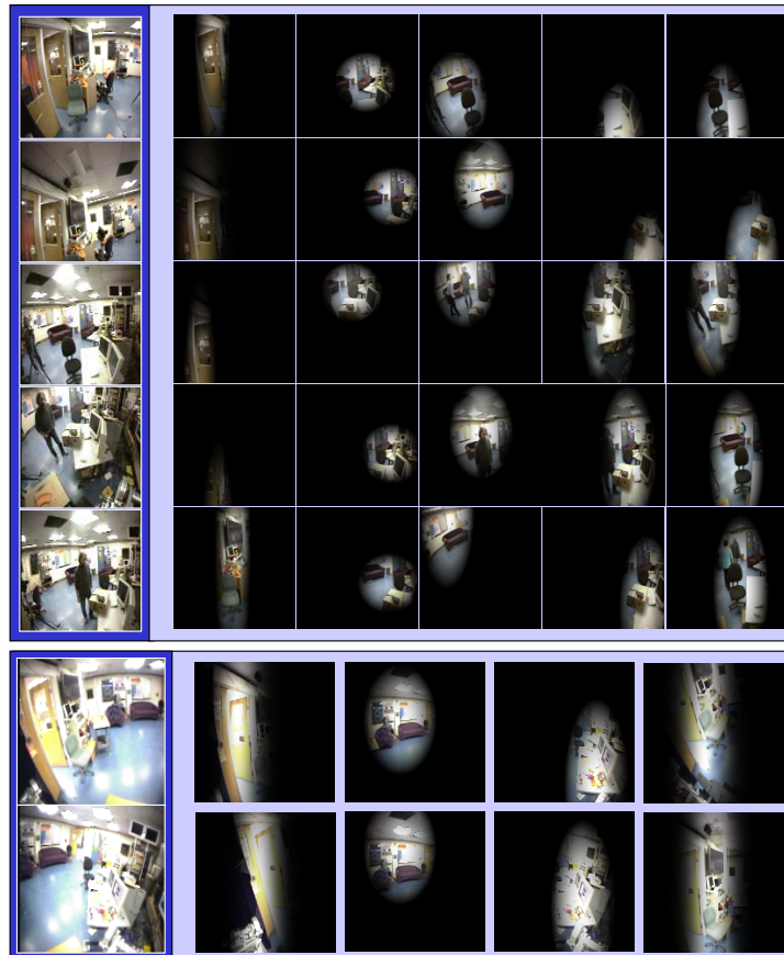
Fig. 8. Localizing and recognizing objects from contextual cues (top) Samples of scene images are shown on the first column. The next five columns show probable locations based on context for finding a door, the smaller sofa, the bigger sofa, the table and the chair, respectively. Even if the object is not visible or present, the system estimates the places at which there is a high probability of finding such object. Two such examples are shown for the chair. Occlusion by humans do not change significantly the context. (bottom) Results in another day, with different lightning.
