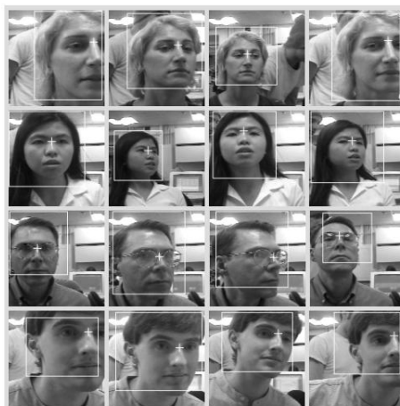
Fig. 9. Eyes are searched for within a restricted part of the robot’s field of view. The eye detector actually looks for the region between the eyes. It has adequate performance over a limited range of distances and face orientations.
