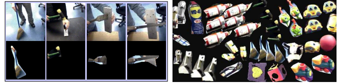
Fig. 5. Samples of object segmentations. (left) Top row shows original images, while bottom row shows segmentations (right) Segmentations from a large corpora consisting of tens of thousands of computed segmentations.
