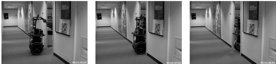
At its full arm extension, with door contact, Cardea's base moves backward slightly, then Cardea moves forward, through the door passage.
