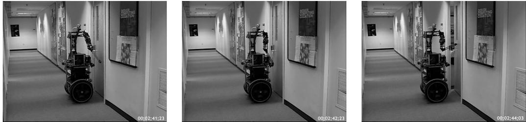
Cardea's fixed action pattern for striking the door. The arm sweeps from its retracted position to the right and downwards then bends up and moves forward.
