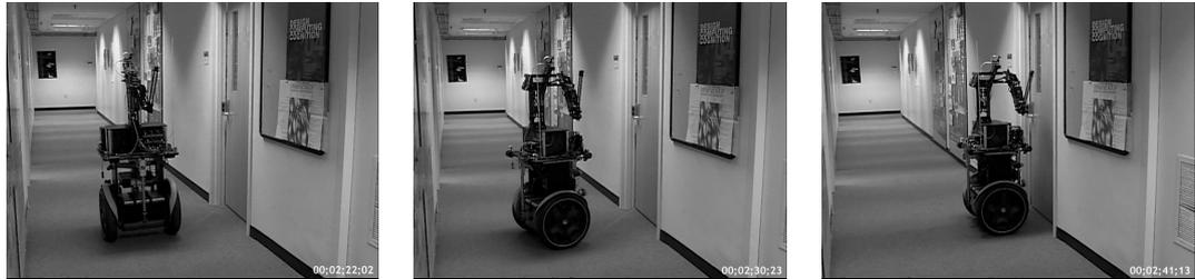
Cardea slows as it first detects the door. Upon confirmation of door, it turns then approaches the door. It adjusts itself to be head on to the door.
