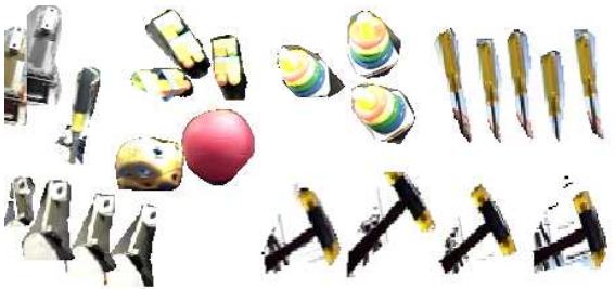
Figure 11. Sample of object segmentations from object's discontinuous motions actuated by humans and the robot. Not only the object's visual appearance is segmented from images, but also the robot's end-effector appearance.
