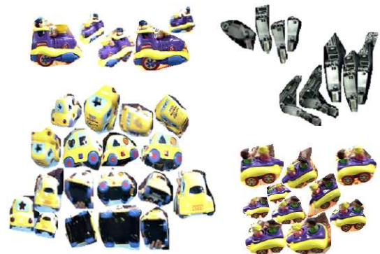
Figure 9. Sample of objects segmented from oscillatory motions, under different views. Several segmentations of the robots arm (and upper arm) are also shown, obtained from rhythmic motions of robot's arm (and upper arm, respectively) in front of a mirror.
