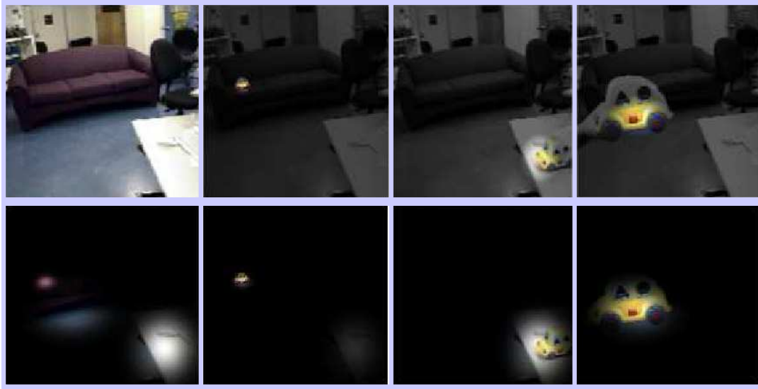
Figure 8-5: The left column shows regions of the image with high probability of finding the car (any size). The next three columns show the regions of higher probability to find the car at a given size scale (smaller, medium and large scales, counting from the left).
