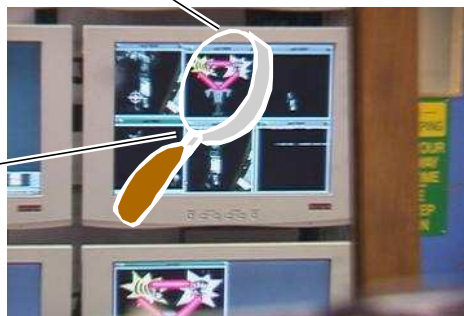
Figure 7-13: In this experiment, Cog is looking at itself in a mirror, while shaking its arm back and forth (the views on the center column are taken by a camera behind the robot's left shoulder, looking out with the robot towards the mirror). The reflected image of its arm is bound to the robot's sense of its own motion, and the sound of the motion. This binding is identical in kind to the binding that occurs if the robot sees and hears its own arm moving directly without a mirror. However, the appearance of the arm (right column) is from a quite different perspective than Cog's own view of its arm.
