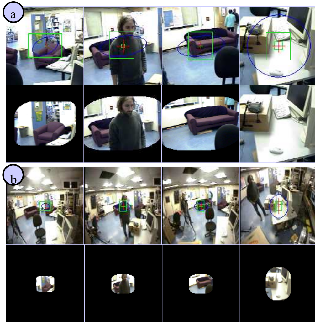
Figure 8-3: (a) Priming object locations. Sample regions (foveal coordinates) computed from predicted size (ellipse) and location (rectangle), plus uncertainties, for objects in a scene. (b) Mapping views. All the data concerning object properties, such as retinal size and location, is mapped onto wide field of view image coordinates, to train the contextual priming system described in chapter 6.
