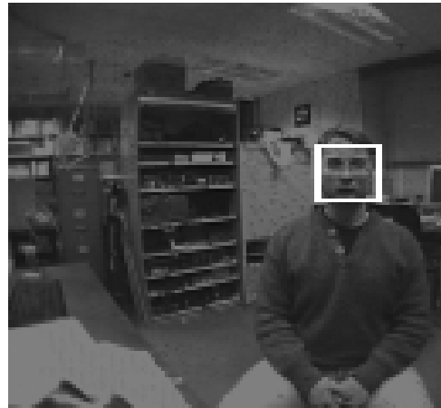
Figure 3: An example of the face detector. The 128x128 grayscale image was captured by the active vision system, and then processed by the pre-filtering and ratio template detection routines. One face was found within the image, and is shown outlined.
