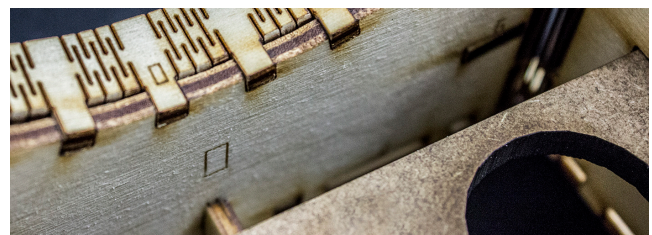
Figure 7: Platener 3D prints/engraves instructions.
