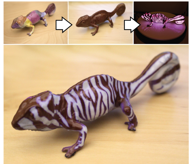
Figure 22. Re-coloring the chameleon (zebra texture) by activating with UV light and applying a new texture.
