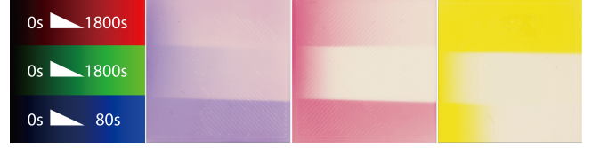
Figure 12. Effect of exposure time of R, G, B projector channels on C, M, Y coatings (left = 0s, with time increasing to the right).
