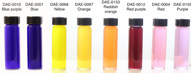
Figure 6. Bi-stable photochromic inks available from Yamada Chemical Co. [22]: 0.1wt% dye mixed in ethyl acetate.
