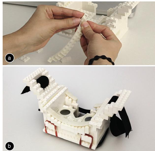
Figure 8: (a) Replacing bricks with the 3D printed parts for the head. (b) The assembled model.
