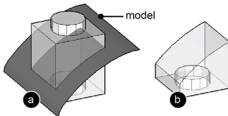
Figure 11: The 3D printable brick is a result of a Boolean intersection of the model and the Lego brick.
