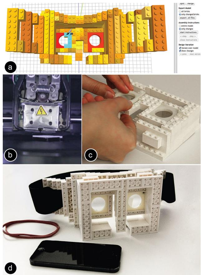
**Figure 1: Let’s fabricate this head-mounted display body quickly: (a) The exact shape of the lens mounts matters; the user thus marks them as “high-resolution” in faBrickator and (b) prints them. (c) faBrickator shows the user how to create everything else from Lego bricks and how to insert the 3D printed part. (d) Done in 67 minutes instead of the 14:30h for 3D printing.**
