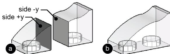
Figure 12: Merging: (a) The sides of each brick are tagged according to their orientation. (b) We use this to identify, which sides need to be removed for merging.
