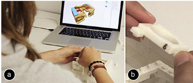
Figure 5: (a) Assembly instructions highlight the next brick in blue. (b) Each 3D printed part has a unique ID.
