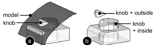
Figure 13: Detecting the completeness of knobs: (a) During intersection, we (b) tag if a part of the knob lies outside the model.
