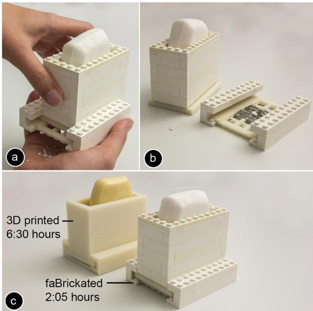
**Figure 14: (a,b) This soap dispenser only takes (c) 2:05h and 5 minutes assembly compared to the 6:30h of traditional printing.**
