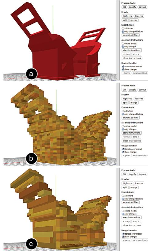
Figure 3: (a) The model is loaded into faBrickator, (b) legofied into 1x1 Lego plates, and (c) layouted.
