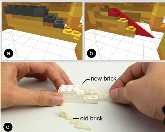
**Figure 9: (a,b) faBrickator highlights what changed between two model versions. (c) The user then reprints only the part that changed.**
