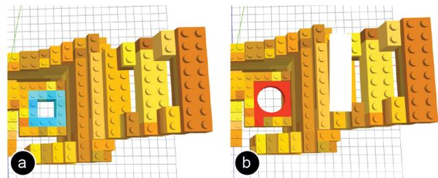
Figure 4: Using the *high-res* brush the user defines the region that will be 3D printed in full detail.
