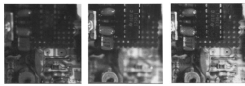
Fig. 9. Multifocus composite image. The original images with limited depth of field settings are shown in (a) and (b). These are combined digitally to give the image with an extended depth of field in (c). Note the values.
