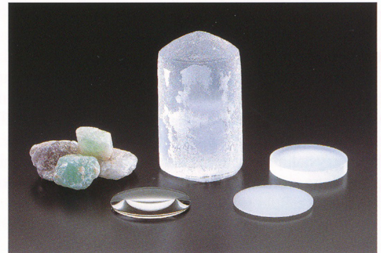
Photo-12 Artificial Fluorite Crystals and Fluorite Lenses
