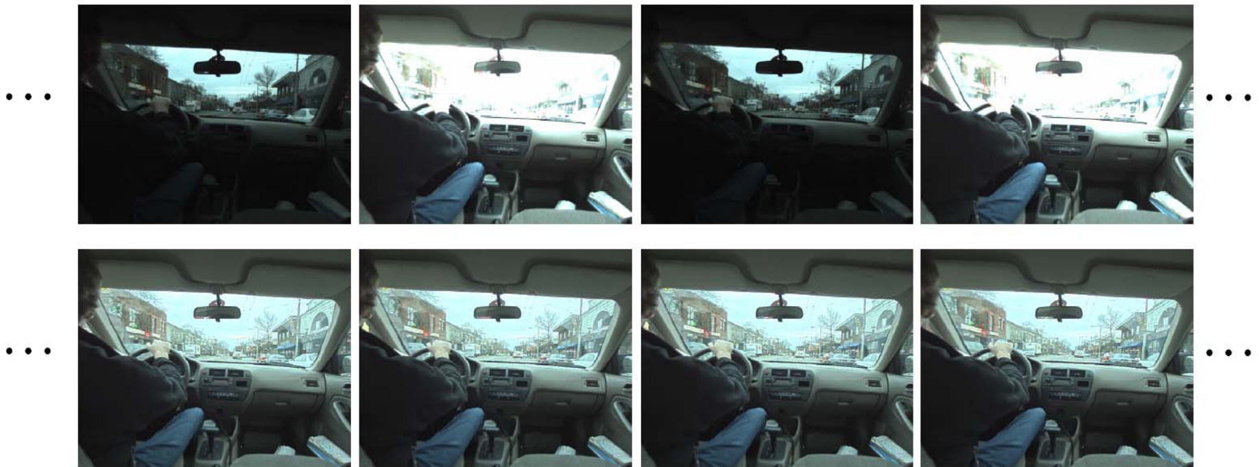
Figure 1: High dynamic range video of a driving scene. Top row: Input video with alternating short and long exposures. Bottom row: High dynamic range video (tonemapped).
