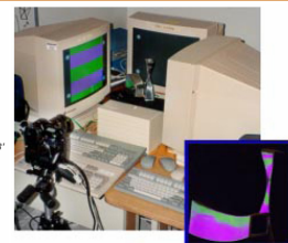
Figure 3 A photograph of the experimental setup used to capture environment matting. The camera is the foreground photograph objects surrounded by overlaid light patterns displayed on the computer monitor. The image is processed to extract only the area covered by the backdrop pattern, resulting in an image as shown in the inset.
