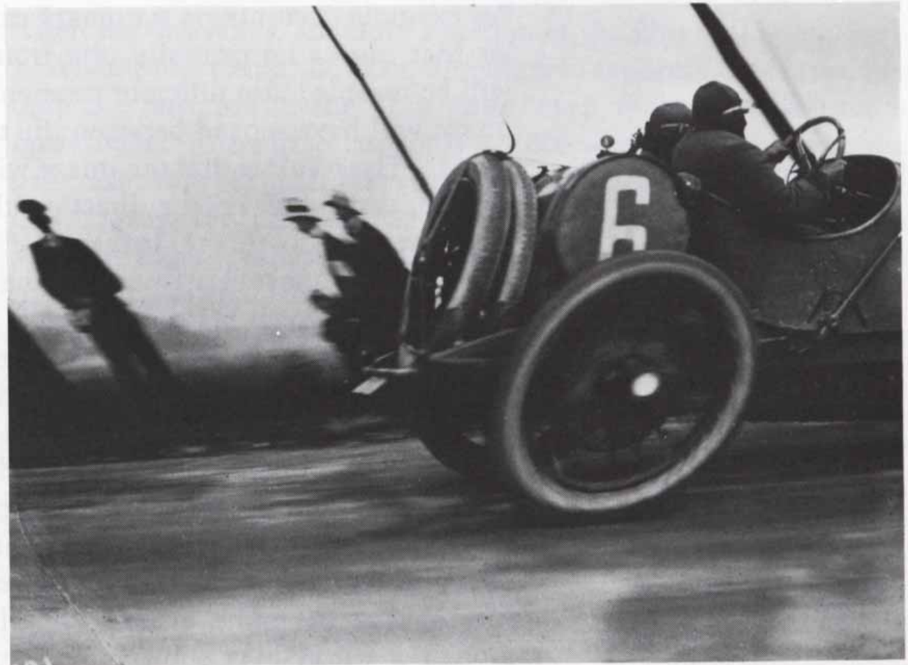
Figure 6–6. Jacques Henri Lartigue, Grand Prix of the Automobile Club of France , 1912. This classic photograph provides an exaggerated example of the distortion that can be caused by a focal-plane shutter. The oval shape of the automobile tire is caused by the motion of the car between the time the bottom of the tire was exposed and the top. (Remember—the image is upside-down on the negative.) The same principle caused the leaning appearance of the spectators. Lartigue turned the camera to follow the automobile (panning), and thus the image of the spectators moved at the film plane during the exposure. (Courtesy International Museum of Photography at George Eastman House.)
