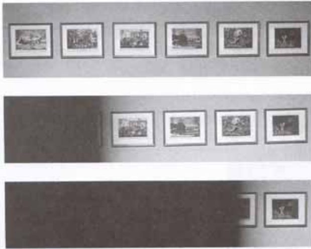
Figure 2-16 Electronic-flash illumination used with a focal-plane-shutter at shutter speeds of 1/60, 1/125, and 1/250 second (top to bottom). At the higher speeds the second curtain begins to cover the film before the first curtain has completely uncovered it. The highest shutter speeds that can be used with electronic flash have increased dramatically with newer single-lens-reflex cameras and flash units.
