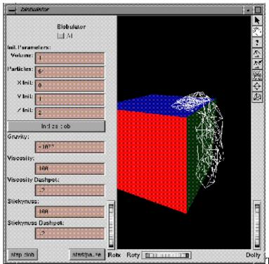
The GUI provides the user with an easy to use interface window that both takes in user input and displays the program output. The window can be functionally divided into two horizontal sections. The left section has a number of input fields that control the parameters of the blob, and the right section is an OpenInventor RenderArea widget that displays a rendering of the blob and its environment. The picture shows a capture of a preliminary blob window.
