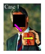
Our PixBlt Method works fine when the source and destination regions do not overlap. But, when these two regions do overlap we need to take special care to avoid copying the wrong pixels. The best way to handle this situation is by changing the iteration direction of the copy loops to avoid problems.
