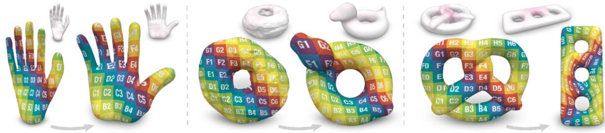
Fig. 1. Visualization of inter-surface maps for pairs of surfaces of varying genus, optimized for low distortion while guaranteeing bijectivity. We represent and optimize such maps flexibly and compactly via discrete constant-curvature metrics of spherical (genus 0), flat (genus 1), or hyperbolic (genus 2+) type.
