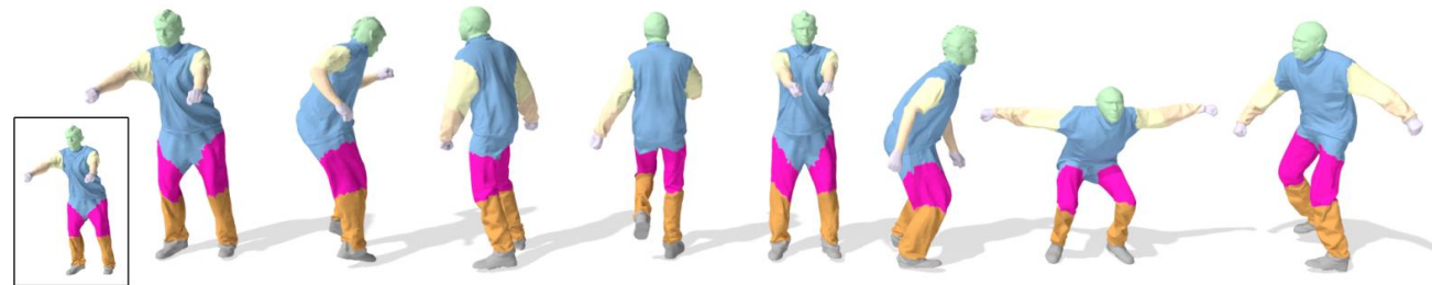
Fig. 1. Mesh segmentation results on the full-resolution MIT animation dataset. Each mesh in the dataset contains 20,000 faces (10,000 vertices). We show an example ground truth segmentation in the bottom-left. In contrast to previous works, which downsample each mesh by more than 10 \times , we efficiently process dense meshes both at train and test time.
